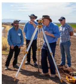
NRAR staff learning field skills. They are using a Dumpy level to measure dam size. Photo: NRAR
