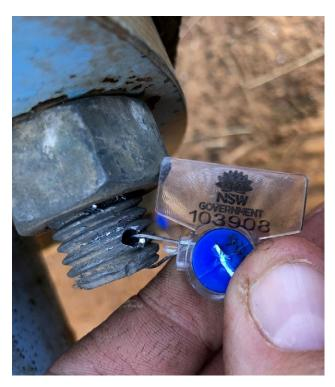
**Figure 3**Example of an installed tamper-evident seal
