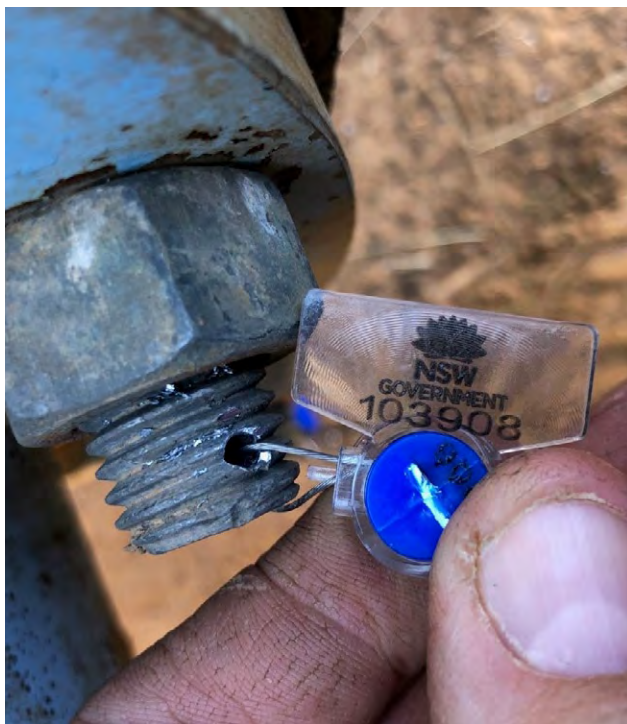
Figure 3 Example of an installed tamper-evident seal
